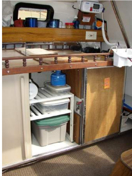
Galley showing stove base. We replaced the original valveless stove with this one which has a valve so that the gas canisters can be removed whenever you want. This also shows the storage above and below counter, Coleman icebox and radio. There is also storage behind the sliding mirrored door behind the counter.
