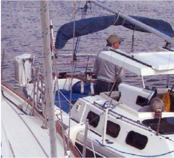
Raft up showing raised pop-top in raised position, Lifesling and Taylor curve-top fender that works well with the R22 flared hull (there are 2 aboard.)
