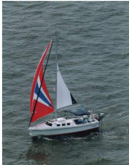
In her slip 2015—you can see the in-mast furling vertical batten main.
