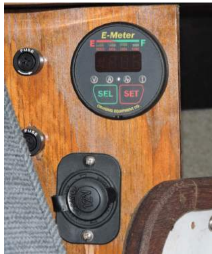
E-Meter (exact same instrument as Link-10, made by the same company) battery and power usage monitor
