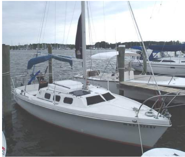
In her slip 2015—you can see the in-mast furling vertical batten main.
