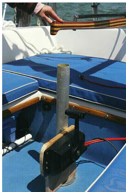
This photo shows the cockpit controls for the outboard mounted to a spare cockpit table leg. We always meant to cut down the leg but found that we liked being able to leave the controls in place and just set the table on top at anchor. We do have another table leg if you would rather set it up without the controls. The whole unit can stow under the seat when sailing to clear the cockpit. You can also see the cockpit cushions and Fretless's unique blue and easy on the eyes cockpit floor.
