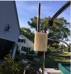
each block. The quote came at \$400! Not in the kitty. Ended up using 2 cutting boards 15" by 20" from WalMart for \$13 each. I had to cut 40 switch plate size wafers that I then drilled using a jig, and joined 2 stacks of 20 with screws and a bolt. I did have to get the appropriate hole saws for \$15 because I had sold
