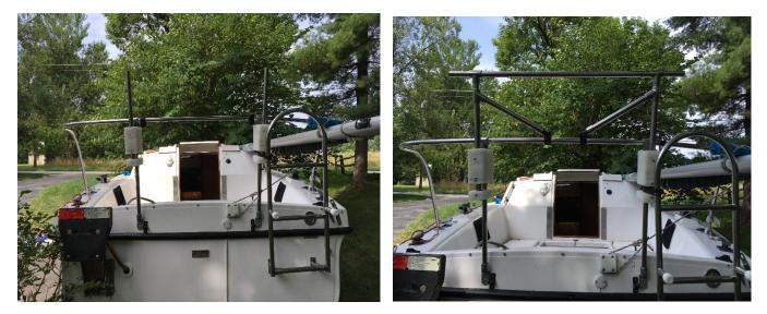
almost all my tools when we moved aboard the boat. Oddly, I did not have to cut a single piece of tubing and use the salvaged fittings to piece much of it together, so no cost there. Each block was then slid onto the aft stanchions by removing them from their base fittings. I then slid the 1" vertical solar supports into
