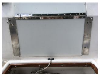
the piano hinge with tamper proof screws, very spendy though. The lock was non-functioning. Steve Jacobs in Washington State had a very robust but simple lock setup but it would make stowing the hatch for me a problem. I order a new lock and installed it; thanks for the info on the list. I also installed a motion alarm in the cabin and a simple contact alarm for the lazzerett. I have never lost anything from the boat but it would be such a pain to try to replace the stuff when I'm overseas.
