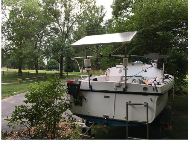
the parallel hole. Finally I drilled through the plastic blocks into the tubing and tapped them with 10-24 thread. I was able to attach some braces the made the whole mount very sturdy. Lastly a cross piece keeps the panel up out of the way and allows the ladder to function. The clamps that have variable friction allow the panel to be tilted. The blocks themselves were salvaged from an old solar array on the big boat.
