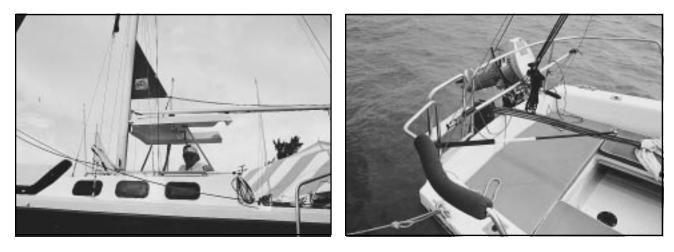
**Above left:** When raised, the pop-top gives 6' 4" headroom below. It is unusual in its use of telescoping supports. When it's down, headroom is about 50". Above right: The mainsheet traveler is a rod extended between the twin backstays—handy to the helmsman, and it cushions the effect of a jibe, but what about wear on the rig?
