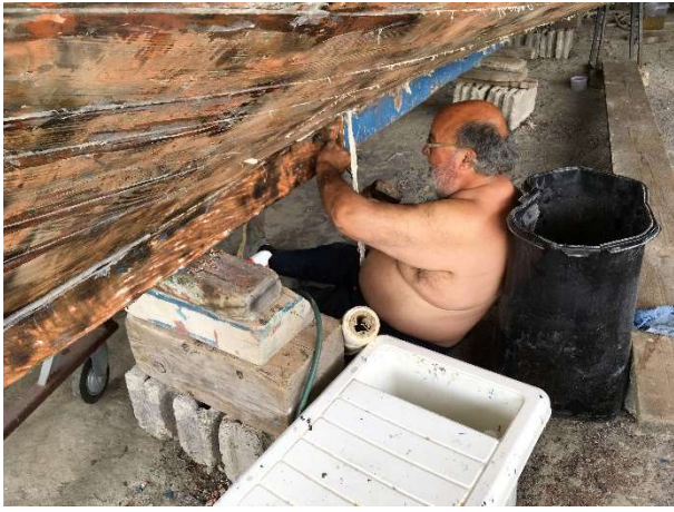
Gianncarlo caulking an old wooden fishing boat.
