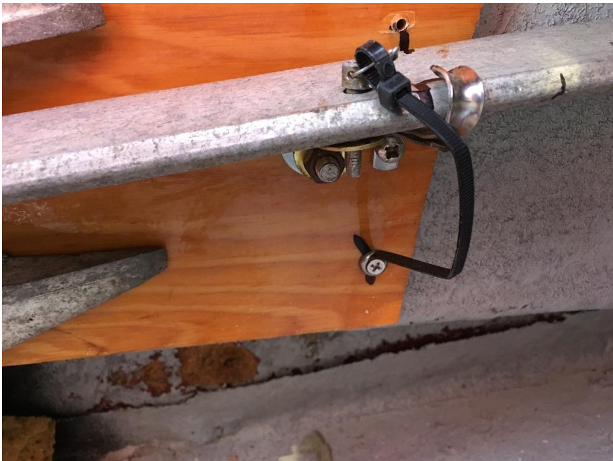
Close up of the locking socket head pin It secures through a hole drilled in the stock to a homemade brass "E" bracket under the stock.
