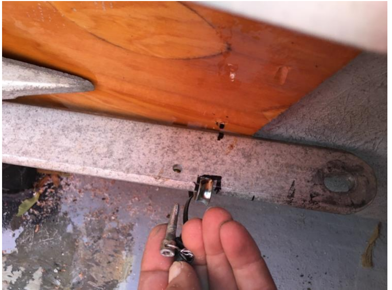
Close up of the locking socket head pin It secures through a hole drilled in the stock to a homemade brass "E" bracket under the stock.
