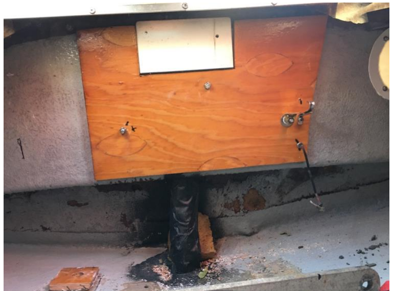
\frac{1}{2} ” marine ply mounted with 3, 5/16 th button head bolts
