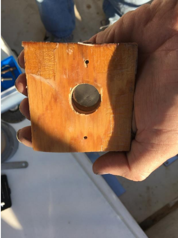
Close up of the base socket for the bottom shank. The backer is an old Schaefer backing plate, secured to the hull by a blob of epoxy putty.
