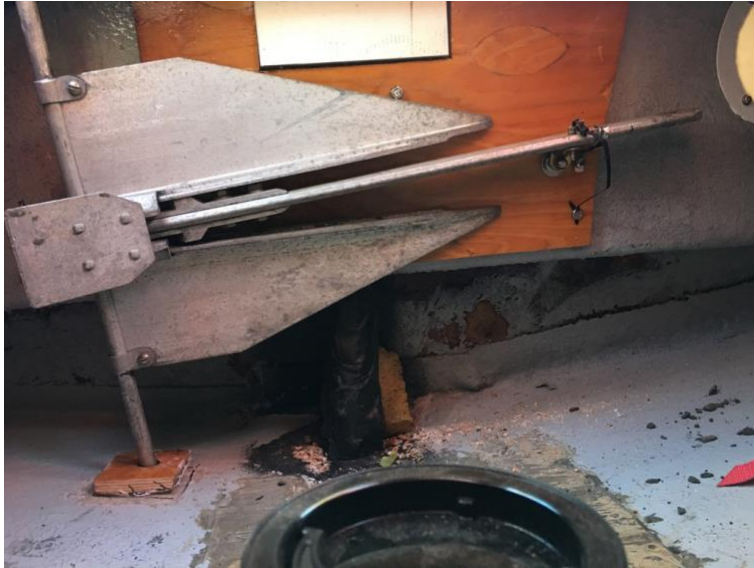
Anchor mounted, top shank is secured by the groove formed by seat gunnel.
