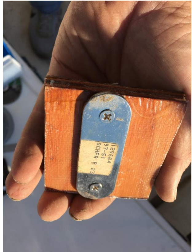
Close up of the base socket for the bottom shank. The backer is an old Schaefer backing plate, secured to the hull by a blob of epoxy putty.
