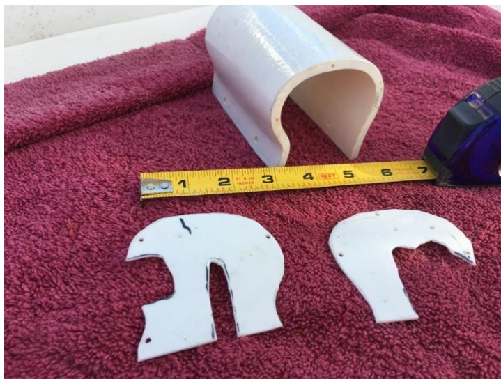
Components took about an hour to make. The end pieces were attached with small Self-tapping screws into predrilled holes.
