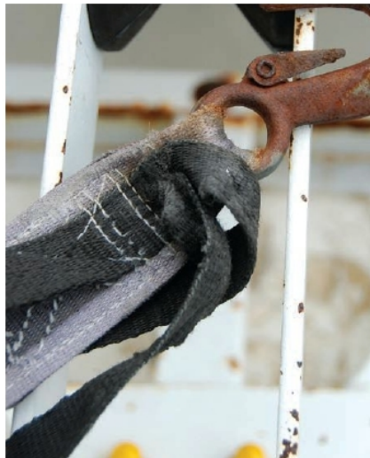
Left: Frayed stitching, tears, cuts, or extreme fading are all signs that the winch strap needs replacement.
