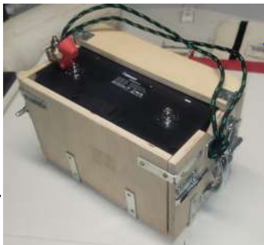
Homemade battery box, nicknamed the Houdini box by my friends. The top piece of wood is on hinges and has clasps to keep it secure.
