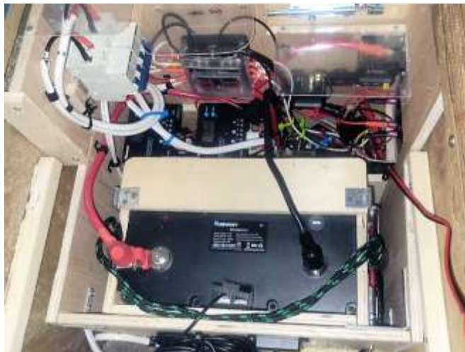
Homemade battery box, nicknamed the Houdini box by my friends. The top piece of wood is on hinges and has clasps to keep it secure.
