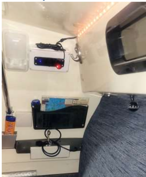
Looking aft, junction box with charger towards port, LED strip. New LED light (not turned on) towards companionway
