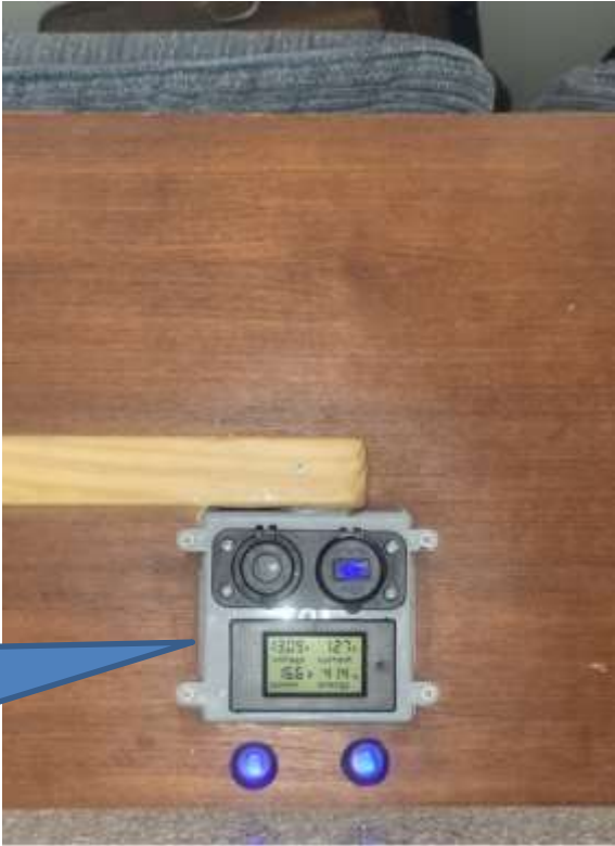
Battery monitor and charging outlets (switches are for the chargers) under fold down bench. Looking forward at bulkhead at aft of v-berth
