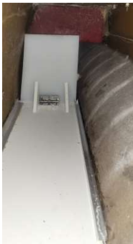
Inside view on port, looking aft. I had to install the back panel on a hinge, then flip it up and add braces
