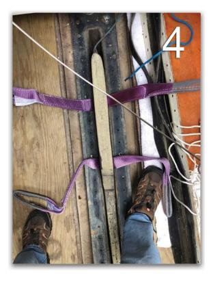
Back to <u>Harbor Freight</u>! I grabbed a chain hoist and used a laughably heavier-than-needed beam I made for something else to lift the centerboard (5-7).
