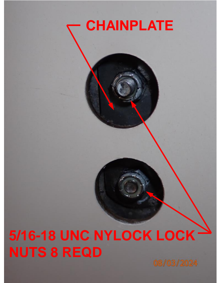
INTERIOR VIEW SHOWING CHAINPLATE & 5/16-18 UNC NYLOCK LOCK NUTS
