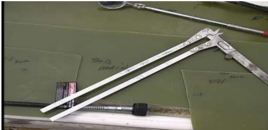
The extended caliper was used to measure the trunk and the middle of the centerboard. Mirrors were essential to seeing into crevices.
